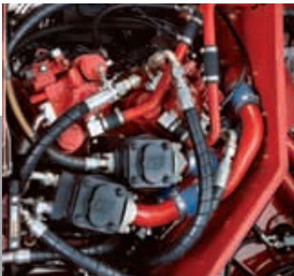
New 3-stage Parker Pump – greater oil flow to the chopper motors.
