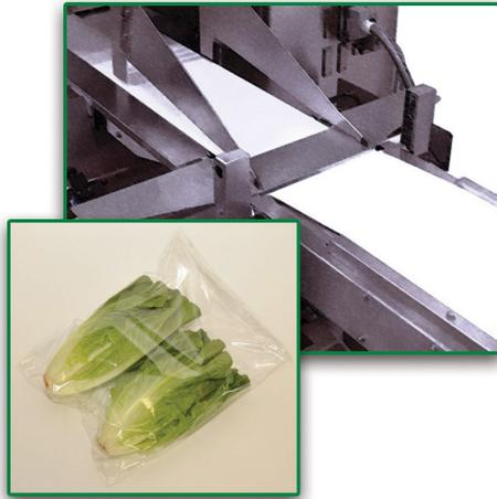
The special feature of this device is the ability to pack products of large dimensions. This machine can package large lettuce, celery bunch, cabbage etc. Also it can even pack small fruits and vegetables in a single unit package.
