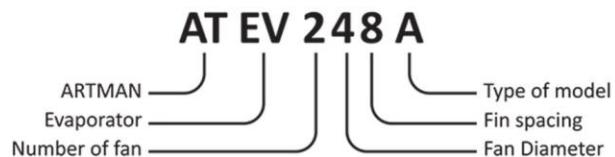
The series ATEV evaporators offer more than 150 different models along with a wide variety of accessories with capacities ranging between 500w , 120 kW
